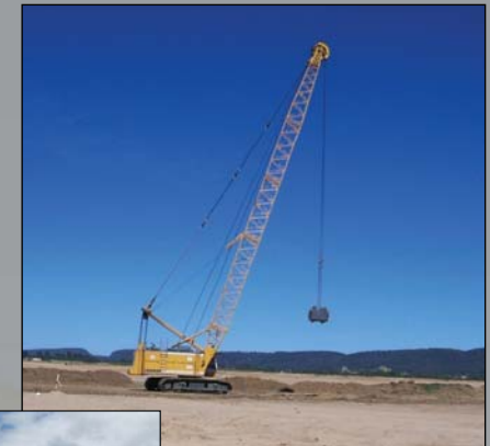
Large crane which will conduct the dynamic replacement
